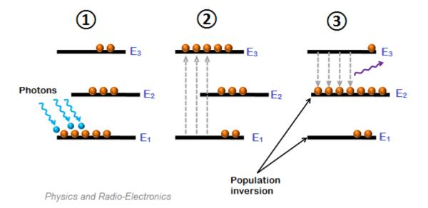
When light energy is supplied to the laser medium (ruby), the electrons in the lower energy state or ground state  $(E_1)$  gains enough energy and jumps into the pump state  $(E_3)$ .
